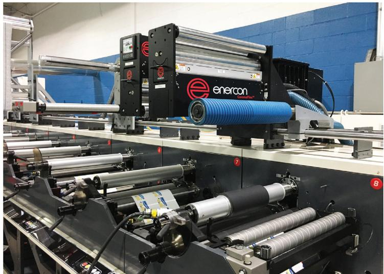
Imburgia says that these materials are some of the most difficult to print on and corona treating is imperative for success. Corona treaters ionize air which imparts surface treatment on the substrates. Treatment increases surface energy and enables print and laminate adhesion. Control Group® relies on corona treatment on almost all of their printing operations. And they specify Enercon Industries for all of their corona treating needs.
